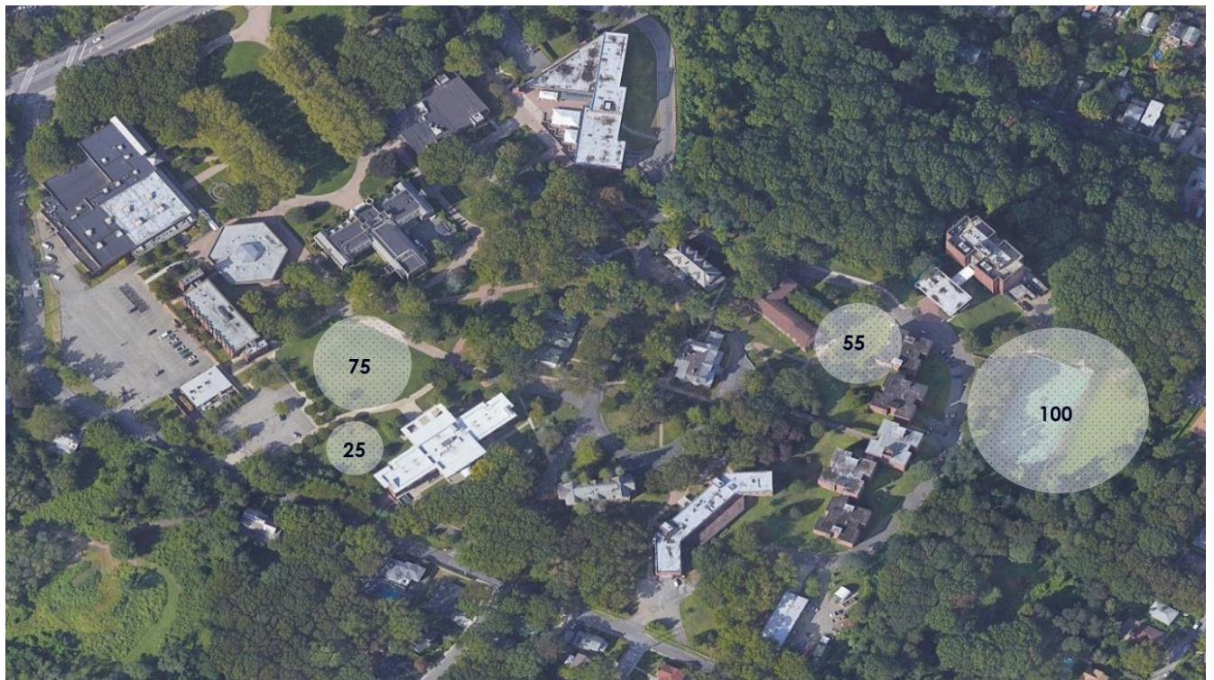
Figure 5. Space Available for Boreholes at Preferred Locations
