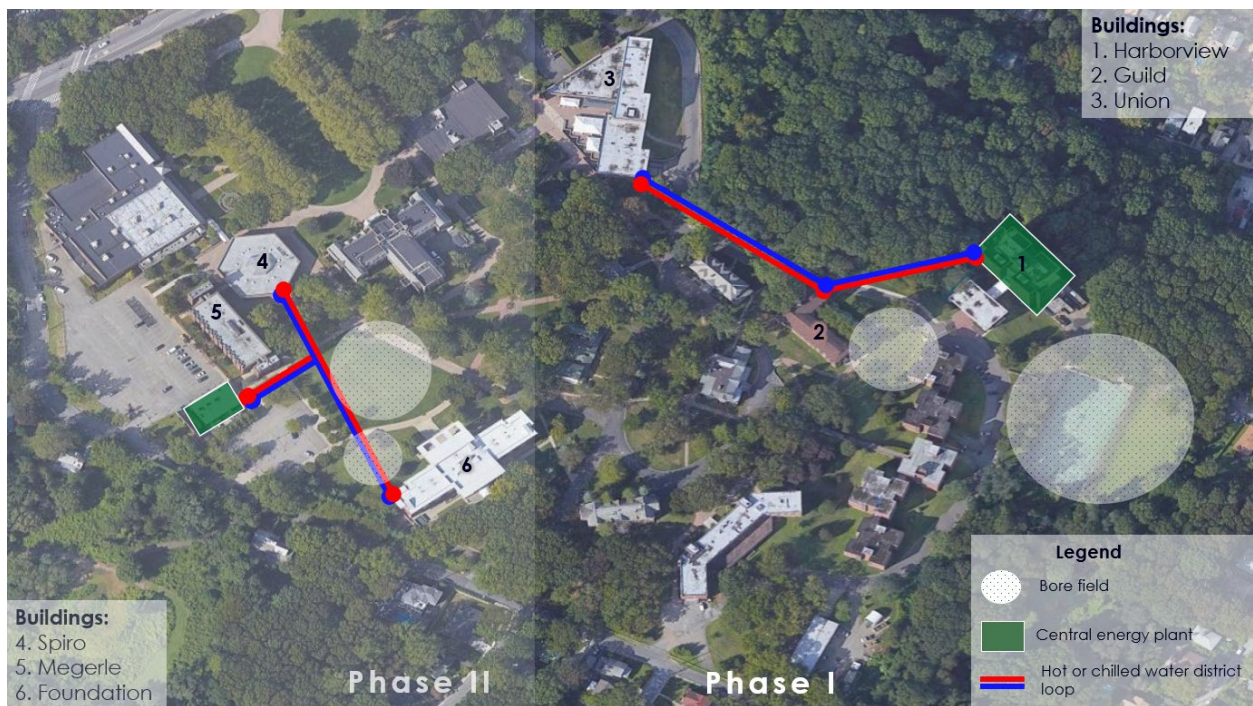
Figure ES-1. Campus Map Showing Proposed Geothermal Districts and Connected Buildings
